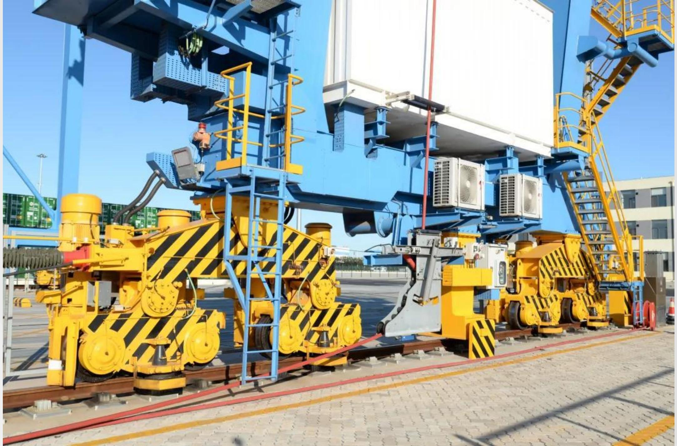
(5) The non-equal-length rear-extension double-trolley bridge crane is first created, which reduces the requirement of foundation bearing capacity and optimizes the layout of bridge crane.
